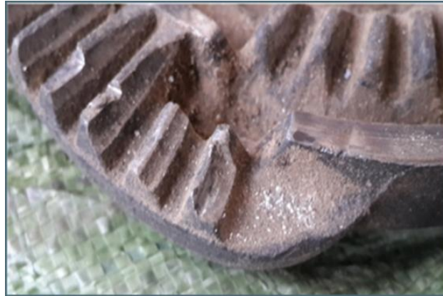
Fig.1 A diagram of damage to the outer teeth
