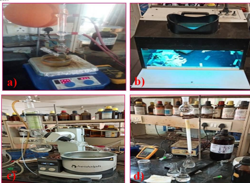
Figure.2. Photograph of a) C-N coupling reaction setup b) UV cabinet c) Rota evaporator d) Celite bed
