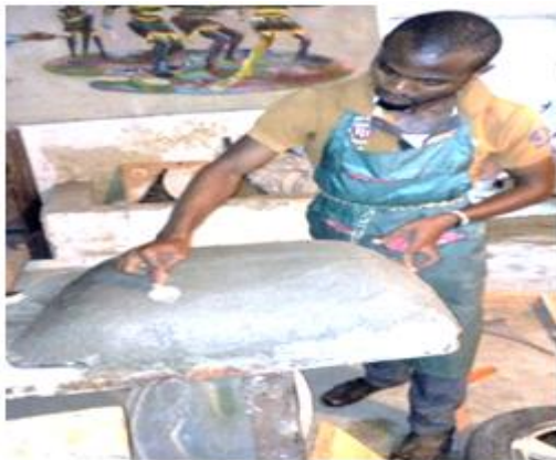
Figures: 4 applying cement on the molded clay
