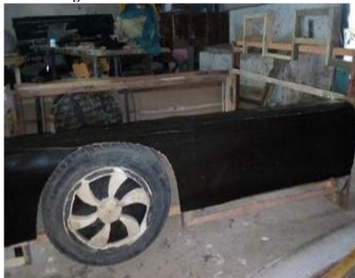
Figure: 8.The tyre with the wood adaptations attached to side rails
