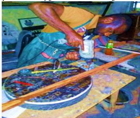
Figure: 6. Screwing and attaching the waste tyre as leg to the configuration
