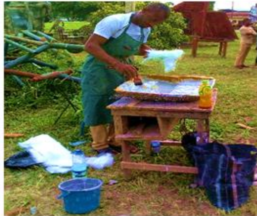
Figure: 5 charging the mold with fibre glass.
